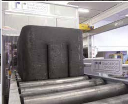
Advanced anodes slotting machines to cut deep, straight, inclined and interrupted slots.
